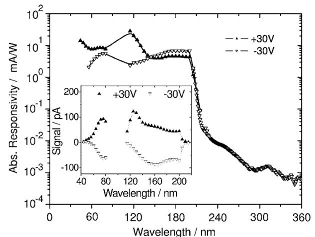
FIG. 3. Absolute responsivity (mA/W) of AlN MSM at  $\pm 30 \text{ V}$  bias between 44 and 360 nm. The inset shows the absolute signal (pA) between 44 and 225 nm.
