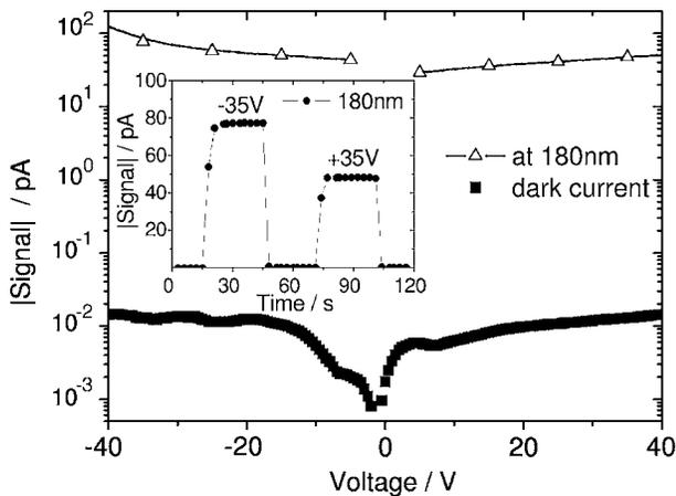
FIG. 2.  $I$ - $V$  characteristics of AlN MSM photodiode at room temperature. The inset shows the absolute signal (pA) as a function of time at 180 nm (400 nW radiant power).
