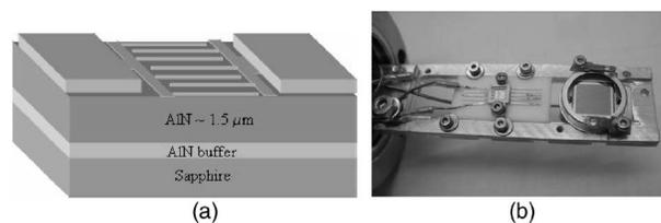
FIG. 1. (a) Schematic representation of the device layer structure and (b) photograph of the AlN MSM photodiode mounted and insulated on a teflon plate inside the manipulation stages holder together with the silicon photodiode reference detector.
